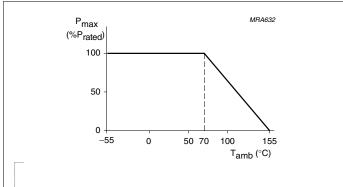
Fig. 5 Maximum dissipation (P<sub>max</sub>) in percentage of rated power as a function of the operating ambient temperature (T<sub>amb</sub>)
