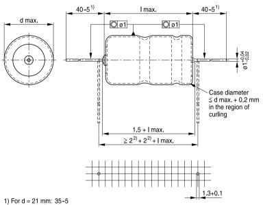
2) Minimum 2 mm bending distance per wire recommended
